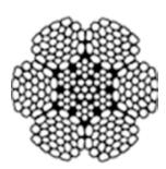
High density construction for greater crushing and abrasion resistance, Greater strength Well servicing rigs must work wherever producing wells need servicing. One of the primary ropes on these mobile rigs is the tubing line.
